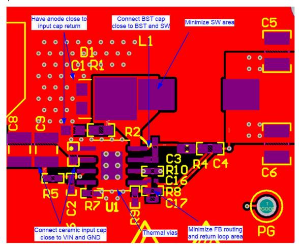
Figure 10-2. LM5013-Q1 Layout Example
