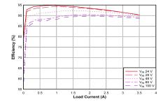
Typical Application Efficiency, V<sub>OUT</sub> = 12 V
