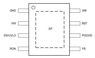
Figure 5-1. 8-Pin SO PowerPAD DDA Package (Top View)
