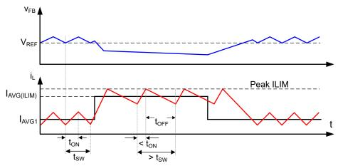
Figure 7-1. Current Limit Timing Diagram
