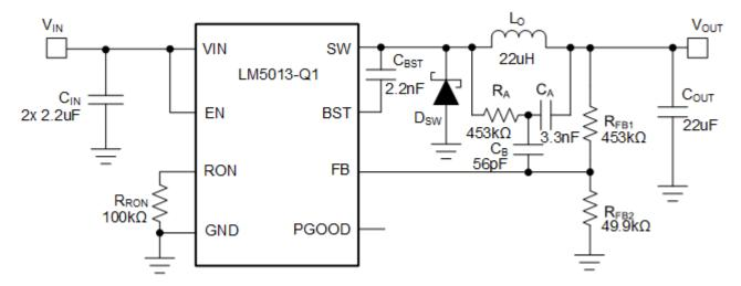
Figure 8-1. Typical Application,  $V_{IN(nom)}$  = 48 V,  $V_{OUT}$  = 12 V,  $I_{OUT(max)}$  = 3.5 A,  $F_{SW(nom)}$  = 300 kHz
