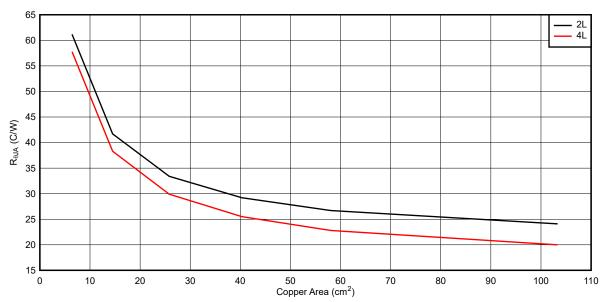
Figure 10-3. Typical R<sub>⊙JA</sub> Versus Copper Area
