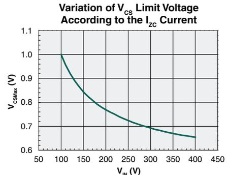
Figure 4.  $V_{CSMax}$  vs.  $V_{IN}$
