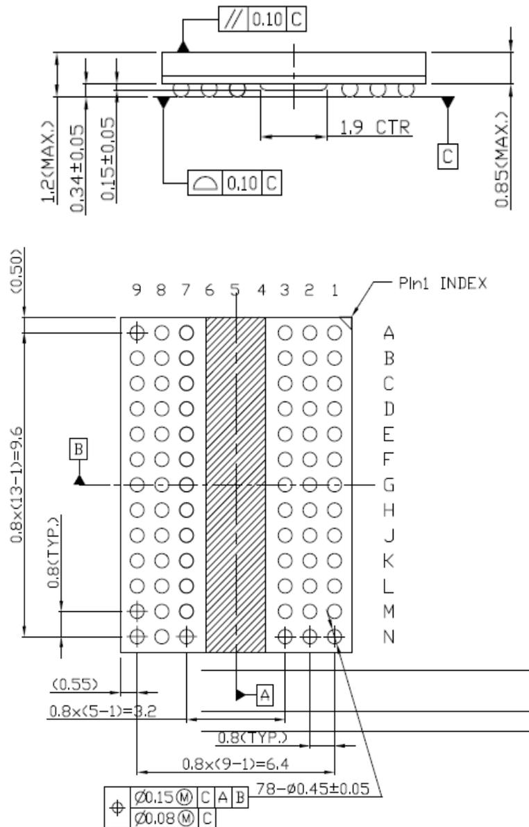
Figure 18 FBGA 78-ball package outline drawing (unit:mm)
