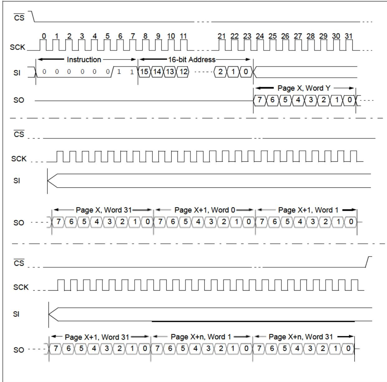
**FIGURE 2-6: SEQUENTIAL WRITE SEQUENCE (SPI MODE)**
