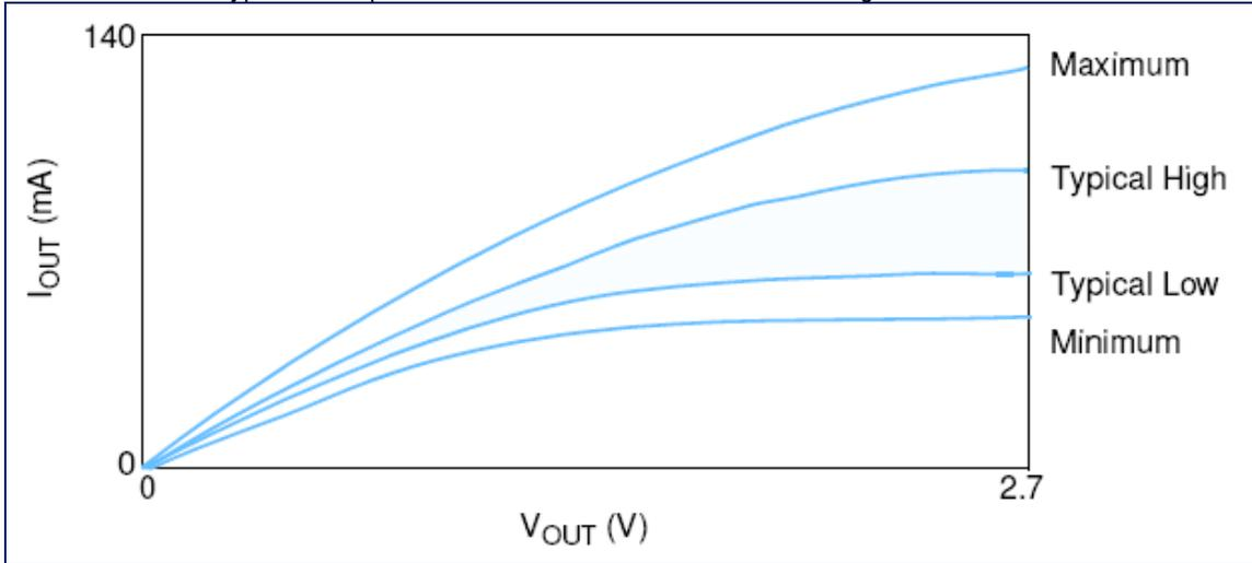
3. The full variation in driver pullup current from minimum to maximum process, temperature and voltage will lie within the outer bounding lines of the V-I curve.
