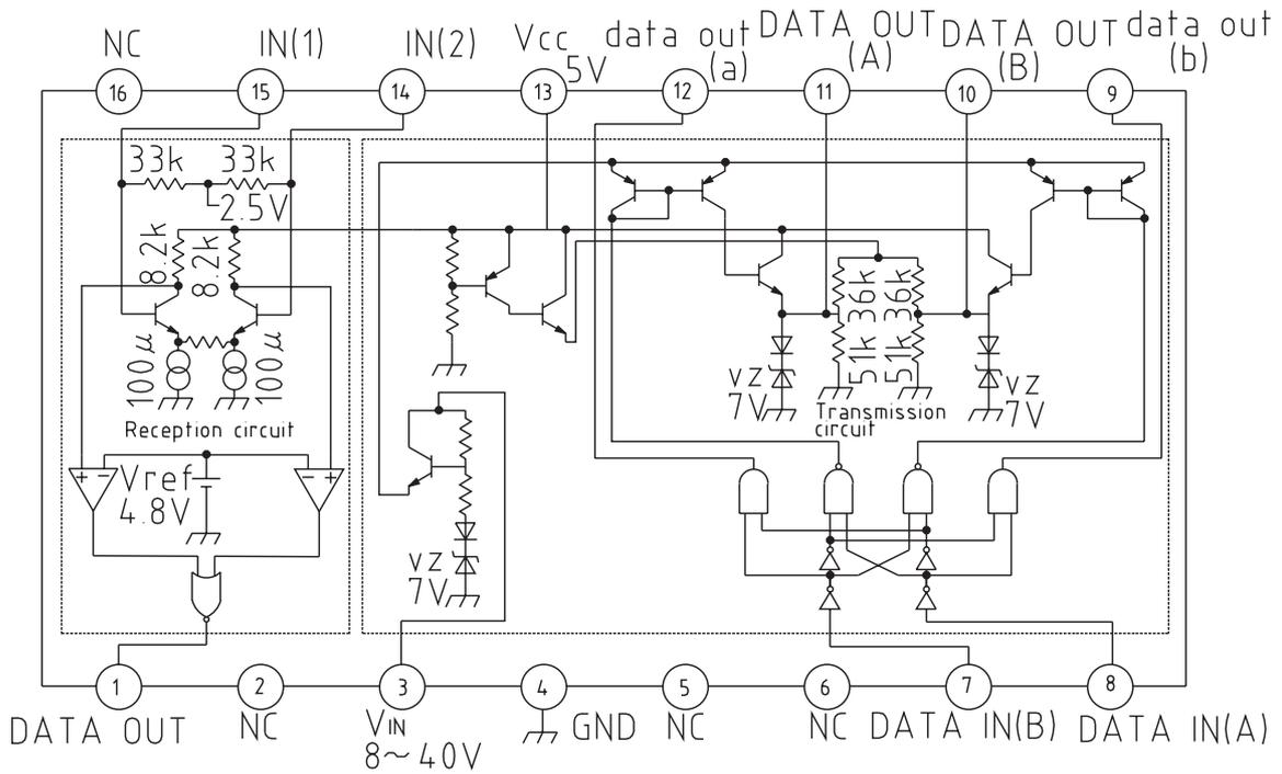
MM1007 When used with a single +5V power supply
