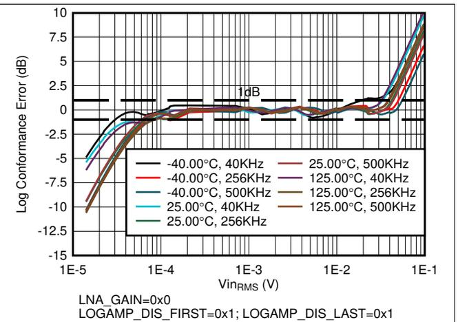
Figure 8. Receive Signal Path Log Conformance Error With First and Last Stage Disabled
