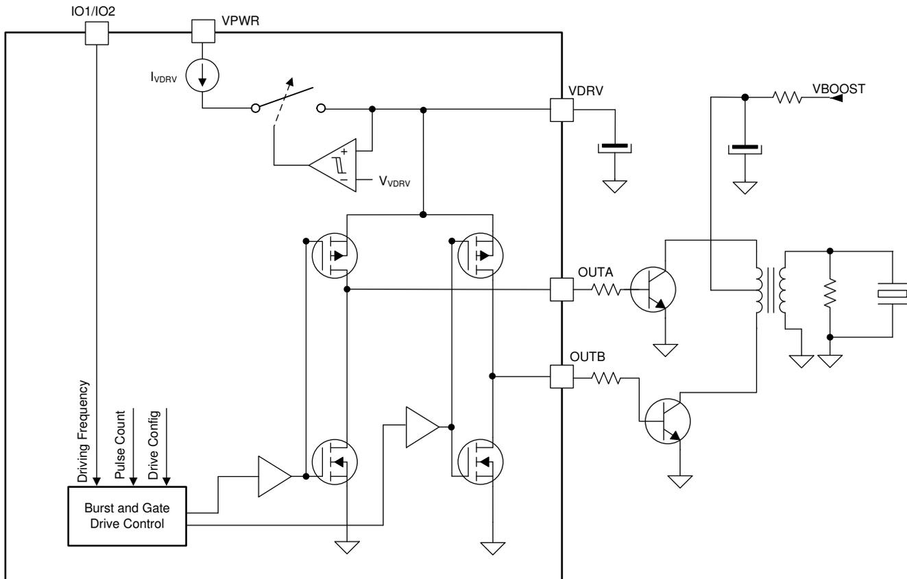
**Figure 20. Center-Tap Transformer Drive Using External FETs**
