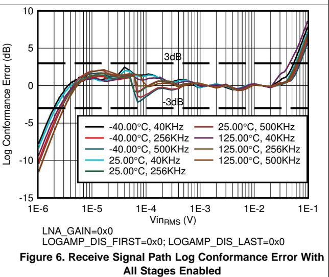
**Figure 6. Receive Signal Path Log Conformance Error With All Stages Enabled**
