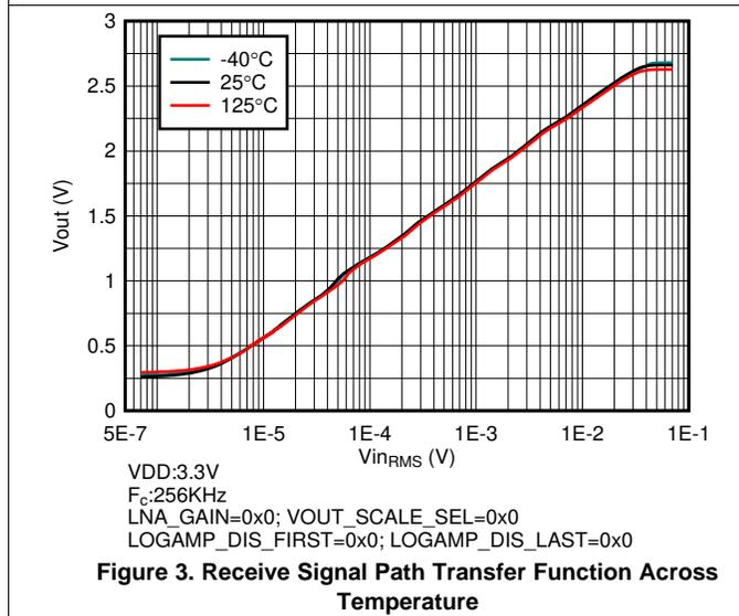
**Figure 3. Receive Signal Path Transfer Function Across Temperature**
