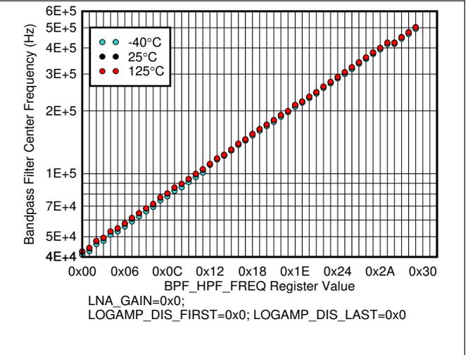
Figure 10. Receive Signal Path Bandpass Filter frequency for Various Register Settings
