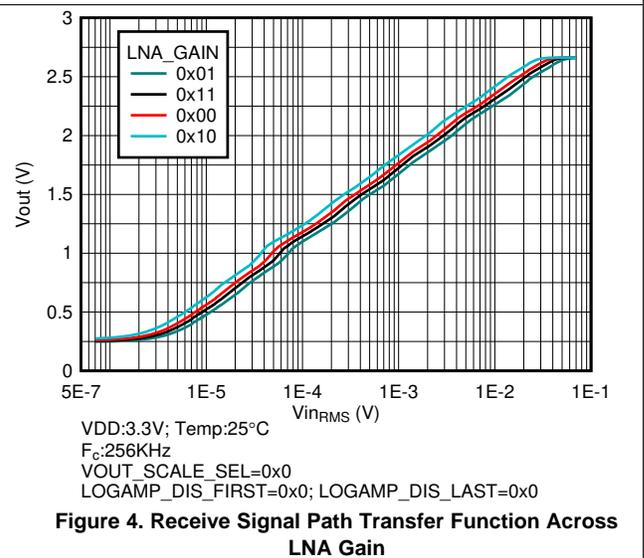
**Figure 4. Receive Signal Path Transfer Function Across LNA Gain**
