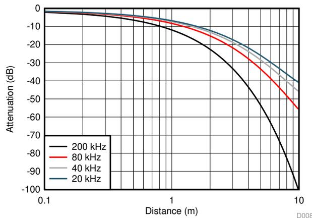
Figure 27. Attenuation Characteristics of Sound Pressure by Distance
