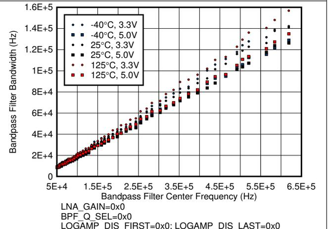
Figure 12. Receive Signal Path Bandpass Filter Bandwidth for Various Center Frequency Settings
