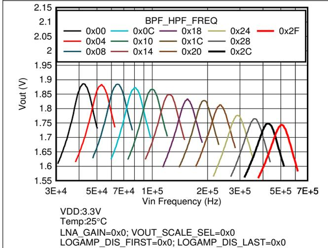
Figure 9. Receive Signal Path Bandpass Filter Transfer Function
