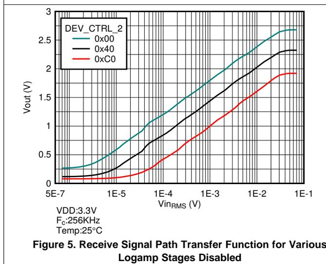
**Figure 5. Receive Signal Path Transfer Function for Various Logamp Stages Disabled**
