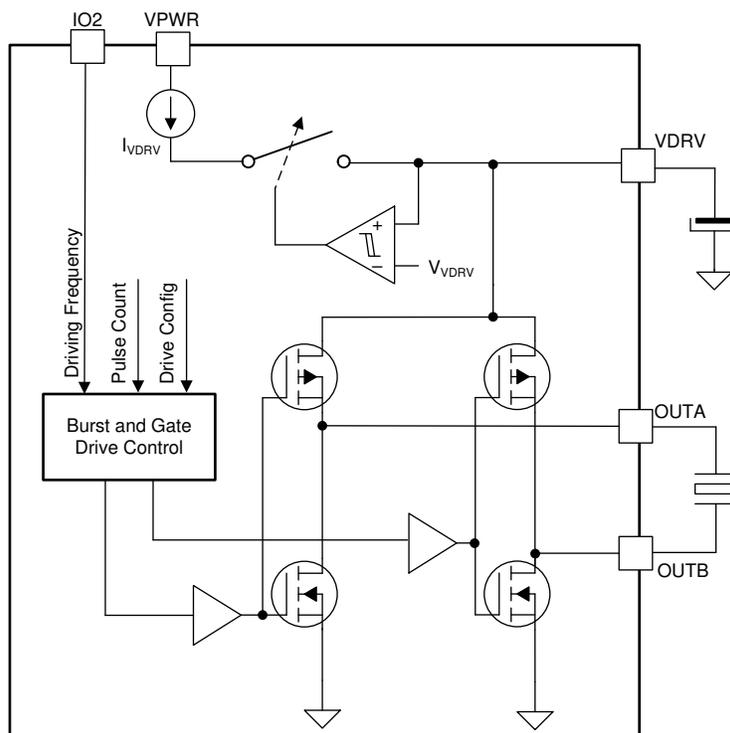
Figure 19. Direct Drive Configuration Using Internal FETs
