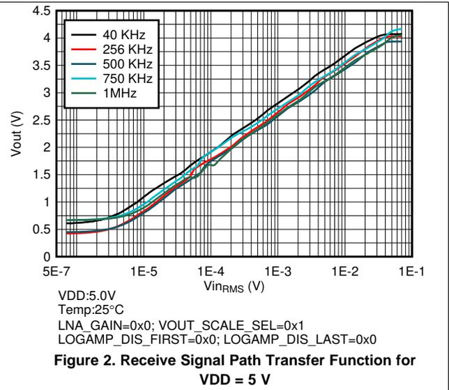
**Figure 2. Receive Signal Path Transfer Function for VDD = 5 V**
