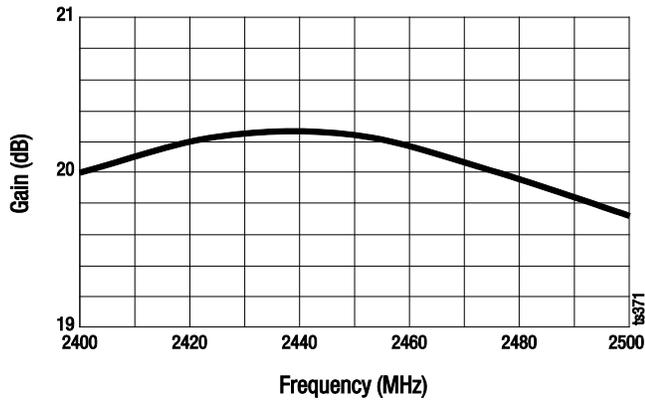
Figure 5. Small Signal Gain vs Frequency, CW
