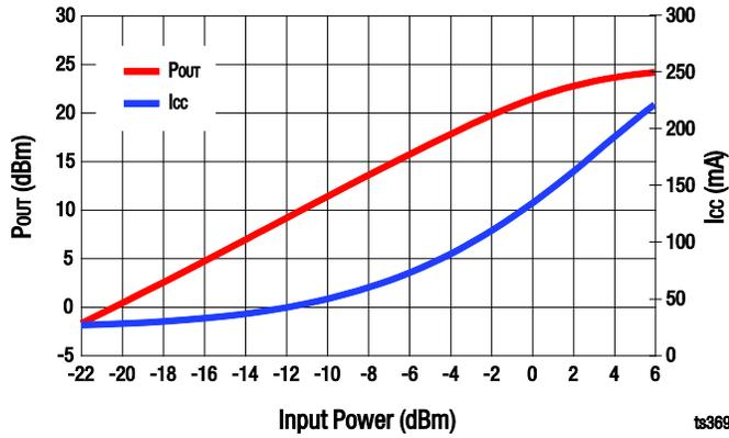
Figure 3. Pout and Icc vs Pin, CW
